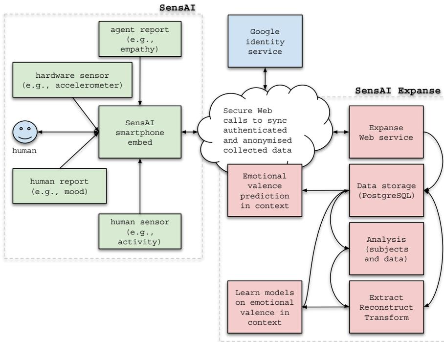
Figure 3.5: SensAI+Expanse data flow.
