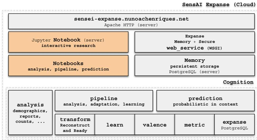
Figure 3.12: The Expense software architecture modules and services.
