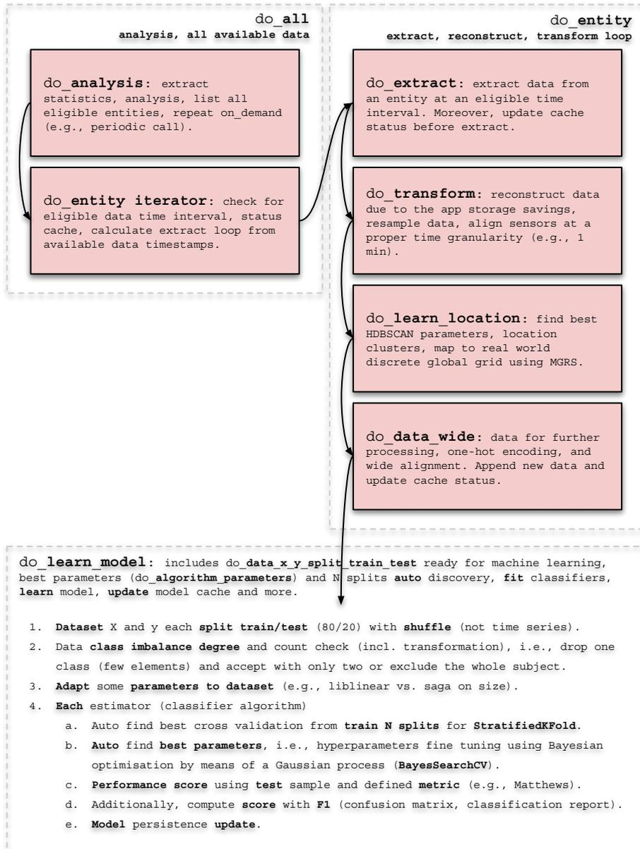
Figure 3.14: Expense machine learning pipeline data flow.
